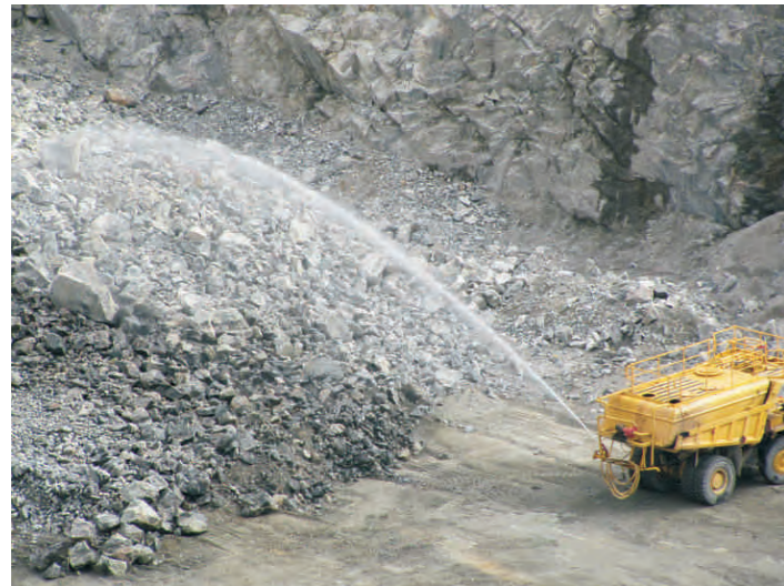
Water truck wetting resource ready for loading and crushing
